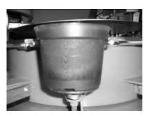
Adjust the pot support height such that the clips of the pot holding disk are a little below the pot edge.
