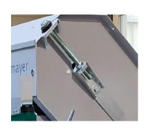
Grease elevator chain prior to a longer shutdown!
