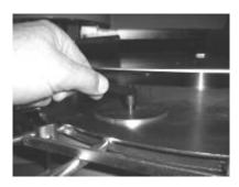
Open the pot receptacle by moving the pot holding disk.
