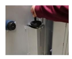
• Adjust soil holder tray with a handle to the height of the pot.
