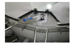
Adjust turntable to place the holder of the potholder disc just under the pot rim.
