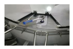
Adjust supports to the diameter of the pot.
