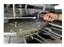
• By means of the reversible ratchet, tighten the adjustable pot holder until the clamps slightly grip the pots.
