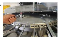
Adjust pot scraper in such a way that excessive soil is scraped from the pot.
