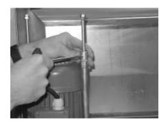
When soft plastic, grided or Jiffy type pots are used, pressing force of the press plate shall be set by using clamping pieces
