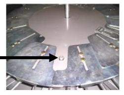
• Adjust soil supports to the diameter of the pots
