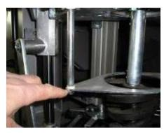
• Set the drilling slide to lower position.
