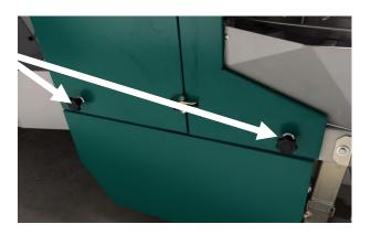
Tight-screw the plate to the holding down bars using selflocking nuts.
