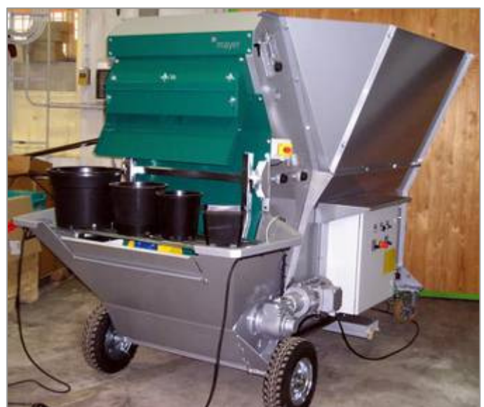
Soil chute for 2 workplaces Different pot sizes can be filled
