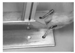
For the dowelling of the machine 4 screws with a minimum diameter of 10 mm and a minimum length of 120 mm should be used with each of the 2 legs.
