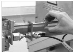
Setting of the distance on the alternating cylinder (performed manually).
