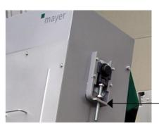
Grease elevator chain prior to a longer shutdown!
