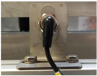
The photo sensor should be set at proper height, so that it can detect incoming pots on the conveyor belt.
